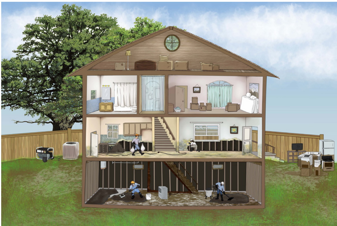
During flood cleanup, completely drying your home and removing water-damaged items are critical tasks.
