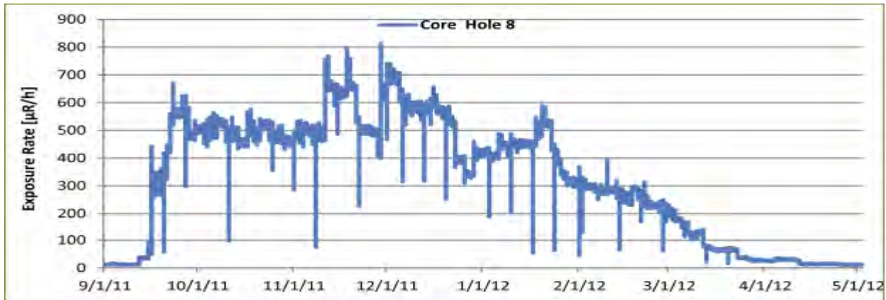
Figure 3: Results of Gamma Exposure Rate Monitoring During the Core Hole 8/Tank W-1A Removal Action (09/01/2011-05/01/2012)
