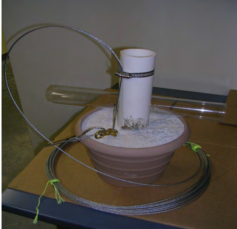
Figure 2: Photo of Sediment Trap
