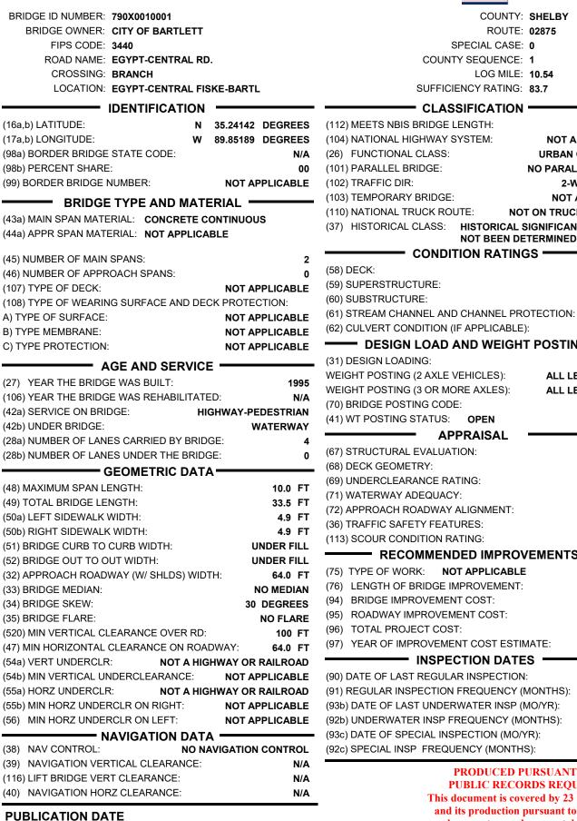
**NO PARALLEL BRIDGE** 2-WAY TRAFFIC NOT APPLICABLE NOT ON TRUCK NETWORK HISTORICAL SIGNIFICANCE HAS NOT BEEN DETERMINED CONDITION RATINGS Ν Ν Ν 6 6 DESIGN LOAD AND WEIGHT POSTING HS-20-44 ALL LEGAL LOADS ALL LEGAL LOADS
