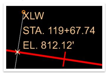
10. With the **Place Node** tool still active, place another node on the other end of the westernmost arbitrary line. Repeat the process to place the remaining 2 nodes. Make sure to key-in the applicable elevation within the **Place Node** dialog box before placement. Once completed, hit **ESC** to clear the tool.
