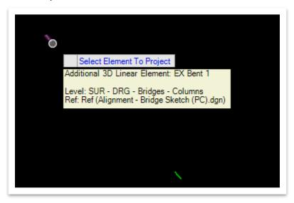
51. Then, turn on the **SUR - DRG - Bridge Deck** level within the active file and select the bridge deck line to project onto.
