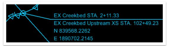
28. Repeat Steps 24-27 to place the downstream intersecting label which will complete the annotation. The corresponding stations should be **6+67.42** and **200+85.55**.
