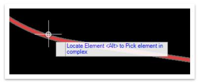
4. Move your cursor to the northern side of the centerline. Left click to accept the placement of the existing ROW line and then left click again to select **Yes to Mirror** so that it is also placed on the southern side.
