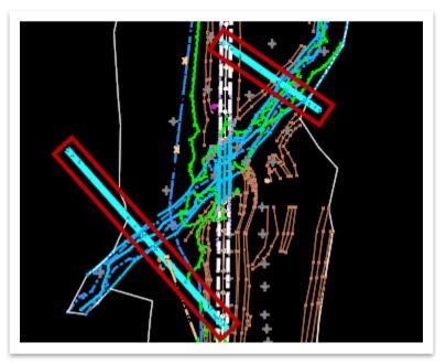
4. Next, we need to extract the creek bed centerline from the reference file into the active file. Open the Plan By 3D Element tool (OpenRoads Modeling >> Model Detailing >> 3D Tools >> 3D Elements). Select the Survey Existing Creekbed Centerline feature definition within the Alignment folder and leave the Name as-is.
