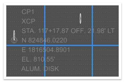
36. Repeat Steps 33-35 to add the label for the other **XCP** conduit. **Note:** As a reminder, the centerline profile does not need to be re-selected before the placement of each label unless the tool was cleared. If ever the station/elevation look erroneous, clear the tool and start again by selecting the centerline.
