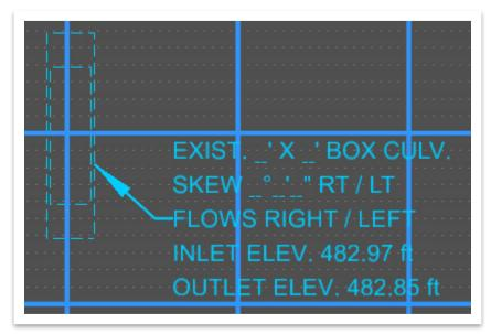
42. Double click within the label to open the **Text Editor** and update the data fields with the applicable survey information, as shown below. **Note:** The data fields have been turned off.
