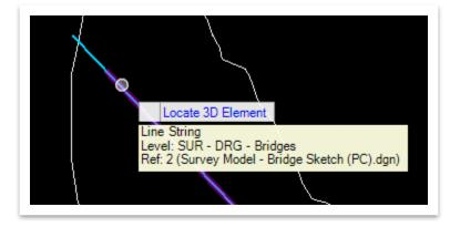
34. Lastly, we will apply the same process to the four bridge column extents. Turn off the SUR - DRG - Bridge Deck and SUR - DRG - Bridges levels in the active file and all reference files for now. The element template was setup on a different level so that the column extents would be easier to see. Then, open back up the Plan By 3D Element tool, if not already opened, and select the Pier/Bent feature definition (Linear >> Structures >> Bridge Sketch >> Existing).
