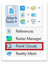
Within the Point Clouds window, go to File >> Attach and select the Knox Co. SR33 Bridge.pod file within the SURVEY\_Training workset dgn subfolder and click Open. Note: For future reference, point cloud Density can be controlled in this window, as highlighted below.
