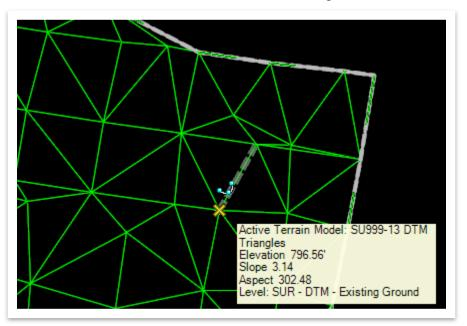
6. Notice that the triangulation automatically updates after deleting the vertex. Hit **ESC** to clear the tool.
