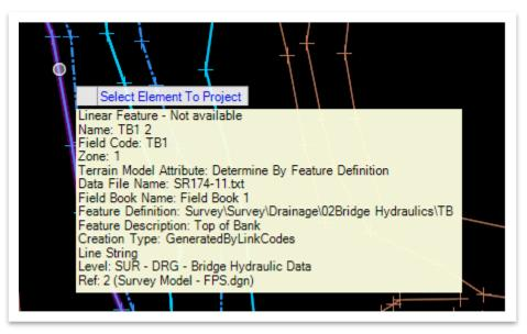
7. Notice the next cursor prompt: **Select Plan Element To Project Onto**. Select the creekbed centerline, as shown below. Once again, prior to selecting the centerline, notice the perpendicular light blue lines indicating the projection region.
