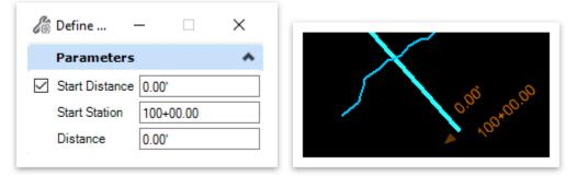
17. Repeat the previous step for the **downstream** XS, except key-in a **Start Station** of **200+00.00**.
