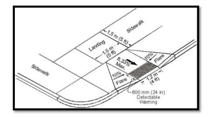
Figure 3 - Curb Ramp Dimensions
