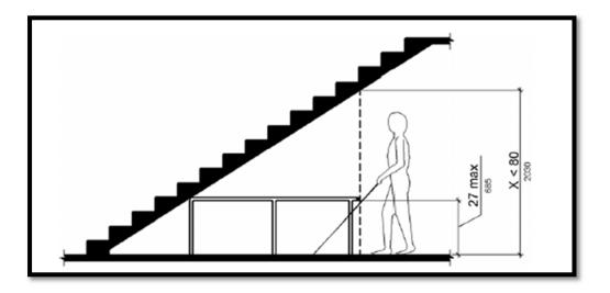
Figure 9 - Suspended Stair Head Clearance
