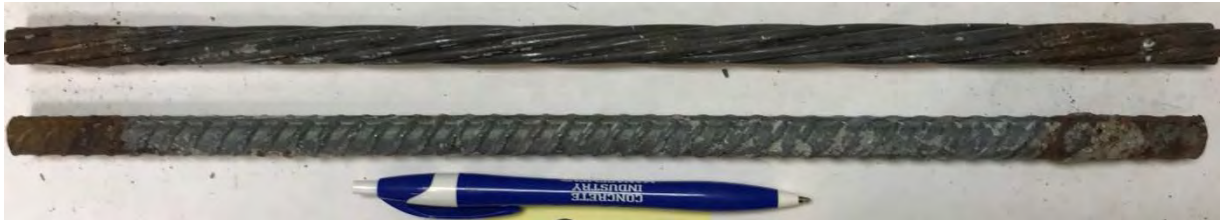
#5-10 (2.0% cast-in NaCl, high-chloride aggregate)
