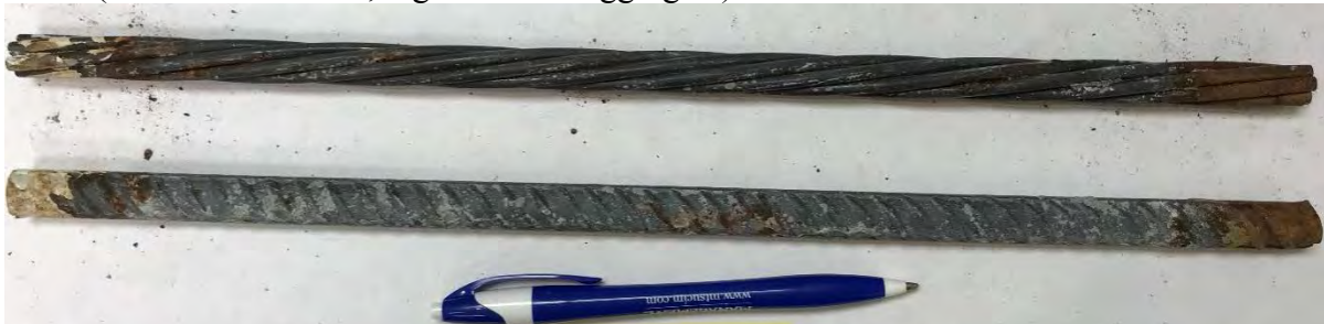
#6-10 (2.0% cast-in NaCl, high-chloride aggregate)
