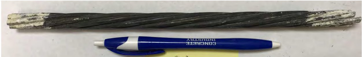
#12-2 (0.3% cast-in NaCl) Unstressed strand
