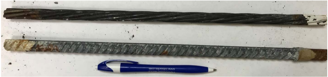
#6-9 (0.3% cast-in NaCl, high-chloride aggregate)
