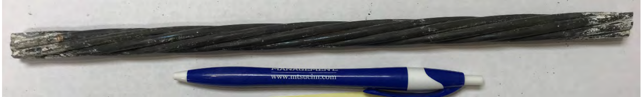
#12-4 (1.0% cast-in NaCl) Unstressed strand
