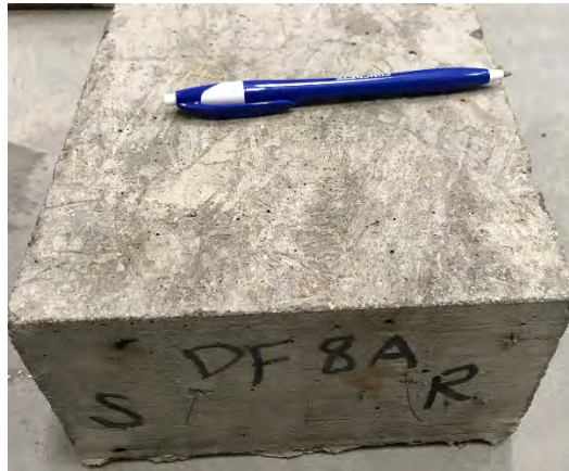
Figure 3.5 An example of concrete slabs for high-temperature exposure
