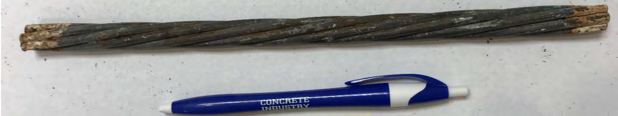
#12-8 (3.0% cast-in NaCl) Unstressed strand
