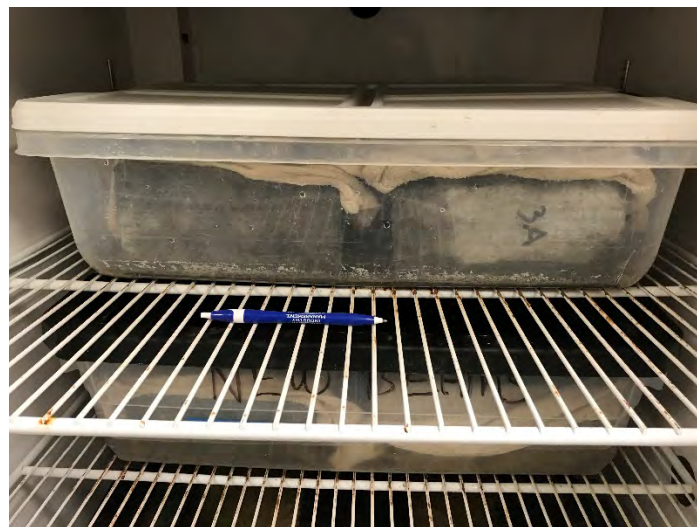
Figure 3.6 Concrete slabs stored at an environmental chamber at 105°F and 50% RH
