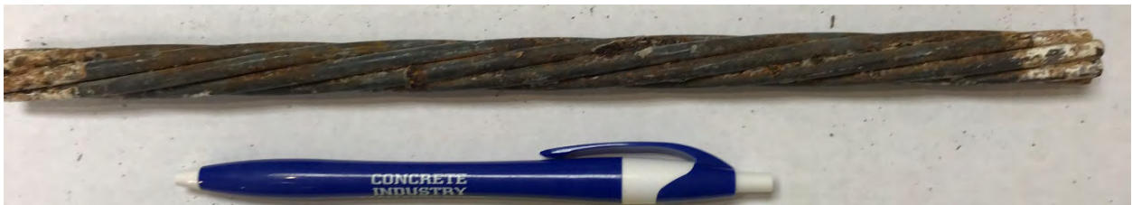
#12-7 (2.5% cast-in NaCl) Unstressed strand
