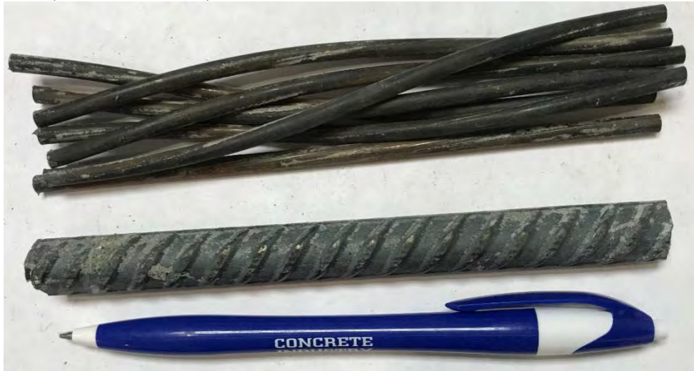
Series 8 - TDOT class D mix, type I cement, high-temperature exposure with moisture #8-1 (0% cast-in NaCl)
