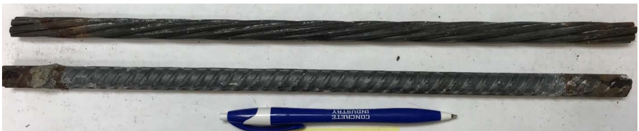
#5-9 (0.6% cast-in NaCl, high-chloride aggregate)
