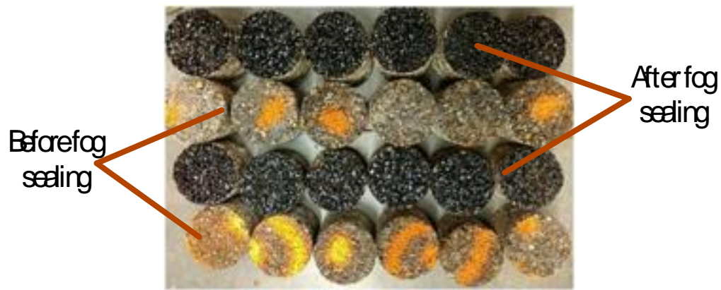
Figure 4-2 OGFC cores with and without fog seal treatment
