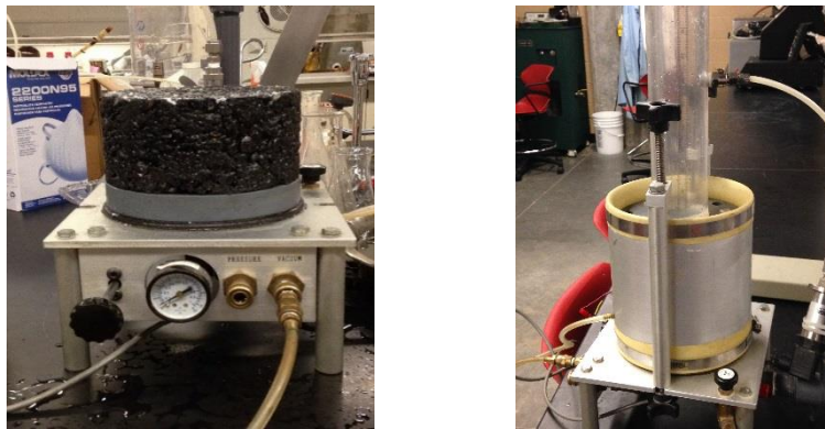
Figure 3-5 Permeability test setup and sample
