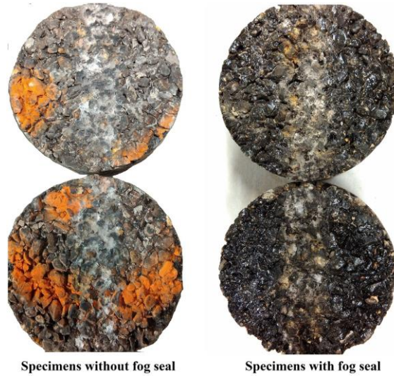
Figure 4-12 Cores after loaded wheel abrasion test
