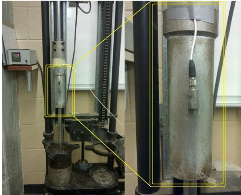
Figure 7-2 Accelerometer installed on the impact hammer
