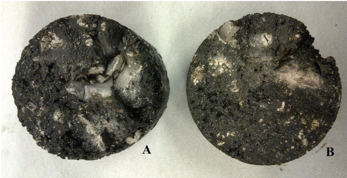
Figure 8-3. Example of the Aggregates damage. (A) Mixture One (307A), (B) Mixture two (307B)
