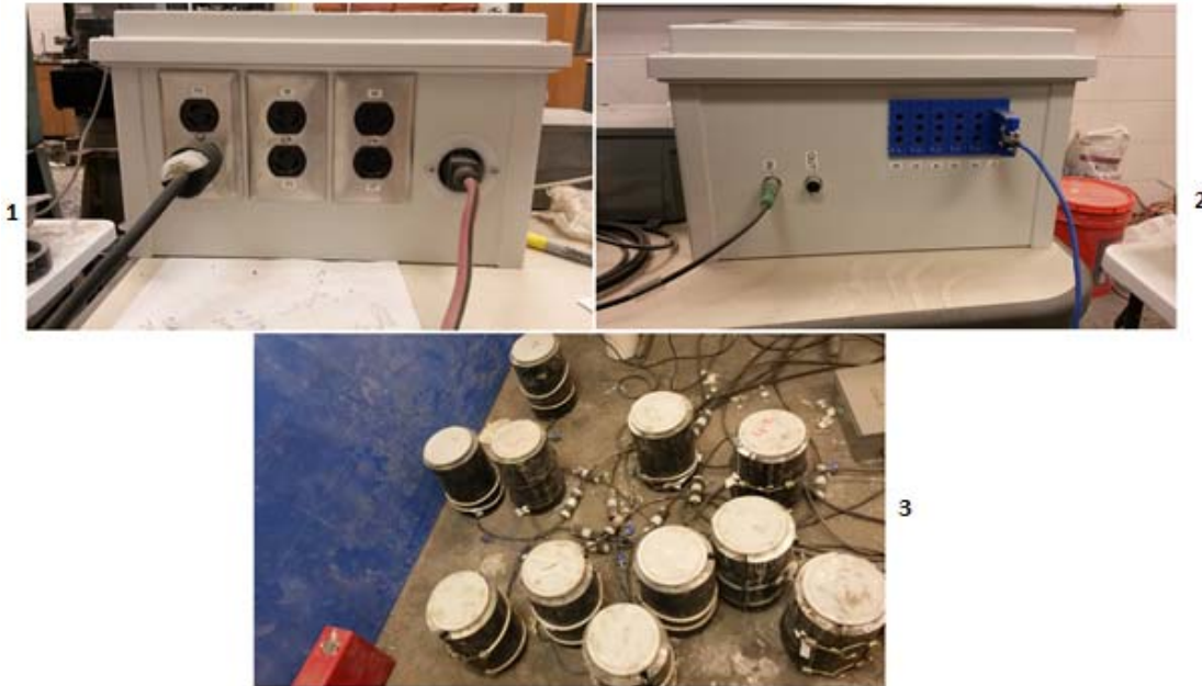
Figure 4.8 SURE CURE System Equipment
