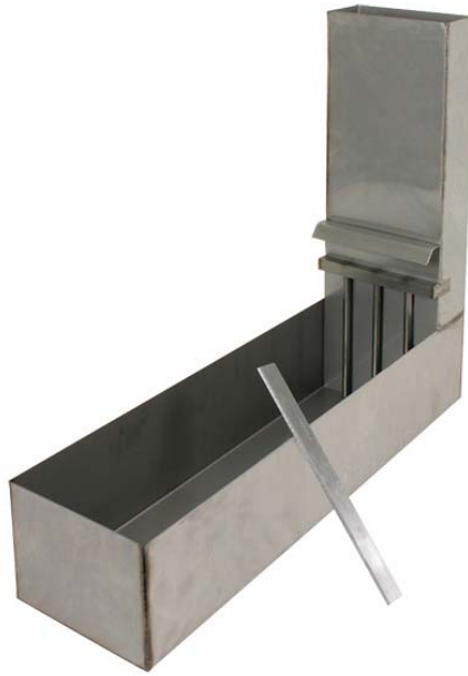
Figure 2.4 L-Box testing apparatus
