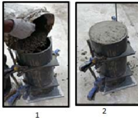
Figure 4.7 The static column segregation
