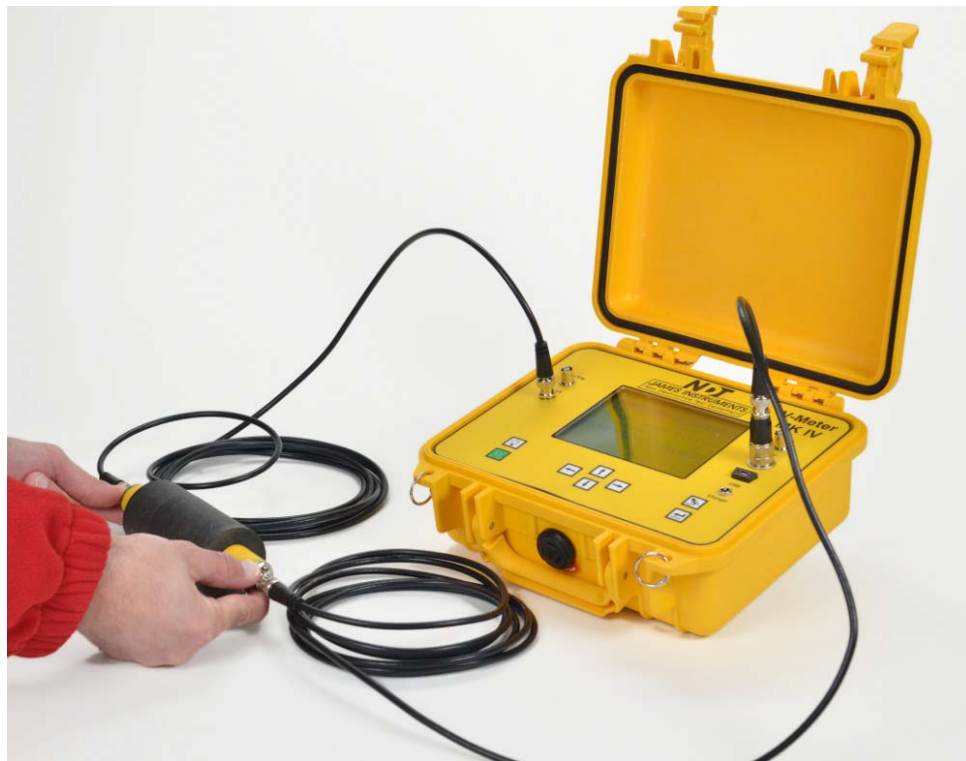
Figure 4.13 Ultra-Sonic Pulse Velocity Instrument
