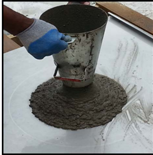
Figure 2.1 Slump flow test
