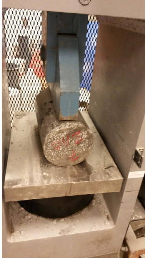
Figure 4.12 Splitting Tensile Strength Test
