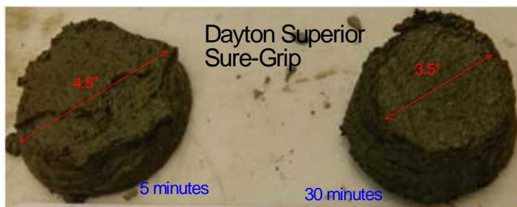
Figure C39 - Spread of mini slump test for Dayton Superior SureGrip Grout at different time at high temperature (95°F) (Mix #5)
