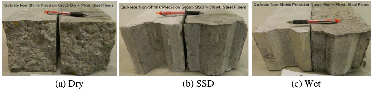
(a) Dry (b) SSD (c) Wet Figure A63 - Failure patterns of flexural bond test for Quikrete Non-shrink Precision grout with 3% steel fiber addition at different substrate surface moisture conditions and normal temperature (73°F) (Mix #14)
