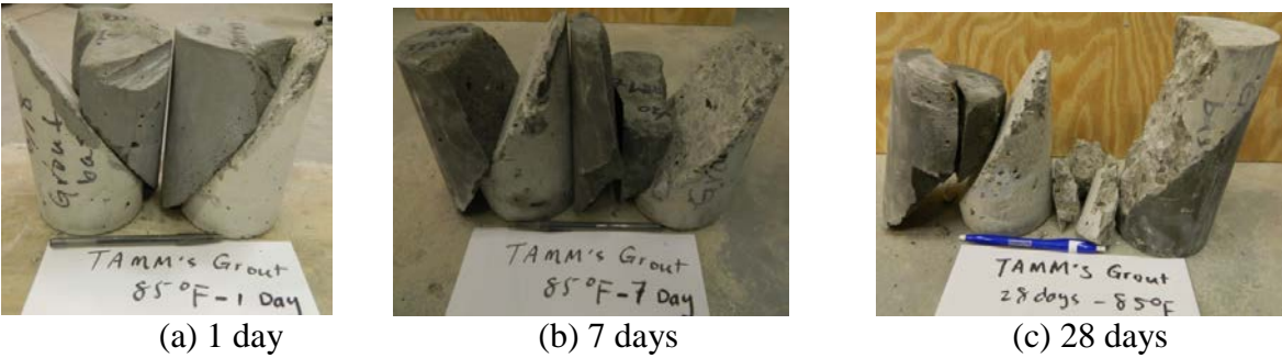
(a) 1 day (b) 7 days (c) 28 days Figure B36 - Failure patterns of slant shear bond test for Tamm's Grout Supreme at different ages at medium temperature (85°F) (Mix #19)
