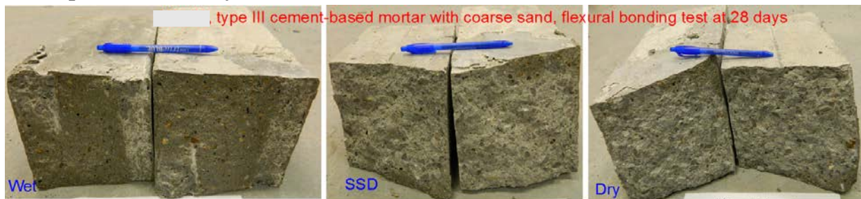
Figure F1-Failure mode of flexural bond test at 28 days for type III cement-based mortar using natural river sand and different substrate surface moisture conditions (#45)
