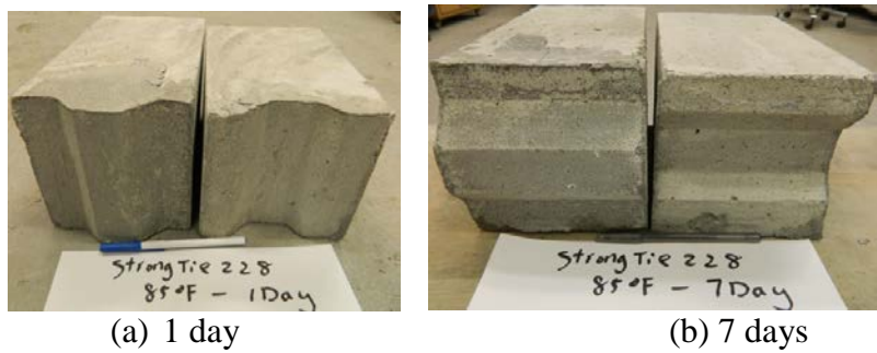
Figure A33 - Failure patterns of flexural bond test for Simpson StrongTie FX-228 Grout at different ages at medium temperature (85°F) (Mix #9)
