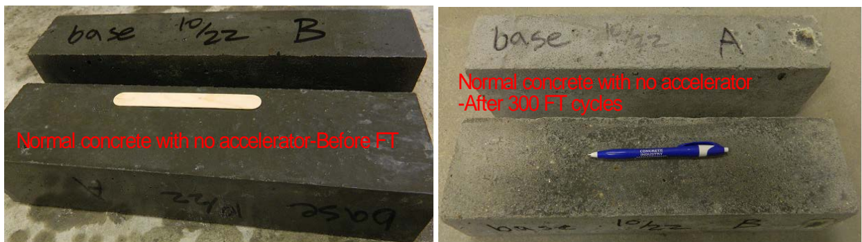
Figure H7-Visual appearance of freeze and thaw test specimens for type III cement-based concrete without accelerator (#53)
