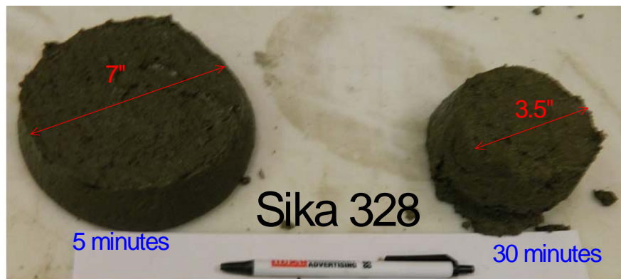
Figure C36 - Spread of mini slump test for Sika 328 Grout at different time at high temperature (95°F) (Mix #2)
