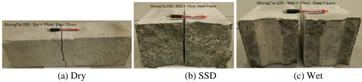
(a) Dry (b) SSD (c) Wet Figure A62 - Failure patterns of flexural bond test for Simpson StrongTie FX-228 with 3% steel fiber addition at different substrate surface moisture conditions and normal temperature (73°F) (Mix #9)
