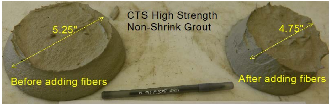
Figure C60 - Spread of mini slump test for CTS Rapid Set CEMENT ALL Grout at normal temperature (73°F) with 3% steel fiber addition (Mix #7)
