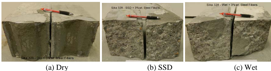
Figure A57 - Failure patterns of flexural bond test for Sika 328 with 3% steel fiber addition at different substrate surface moisture conditions and normal temperature (73°F) (Mix #2)
