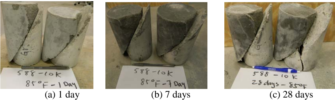
Figure B31 - Failure patterns of slant shear bond test for W.R Meadows 588-10K Grout at different ages at medium temperature (85°F) (Mix #6)
