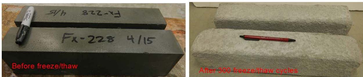
Figure D8- Visual appearance of specimens before and after freeze and thaw test for Simpson StrongTie FX-228 (Mix #9)
