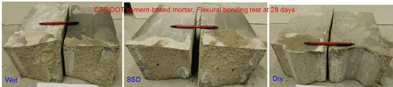
Figure F10-Failure mode of flexural bond test at 28 days for CTS DOT cement-based mortar with different substrate surface moisture conditions (#55)
