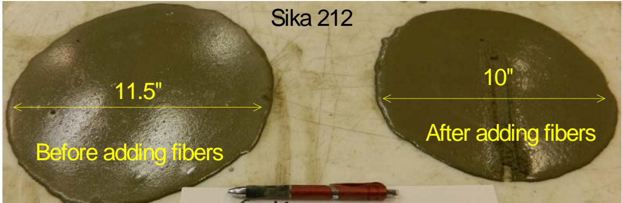
Figure C57 - Spread of mini slump test for Sika 212 Grout at normal temperature (73°F) with 3% steel fiber addition (Mix #3)
