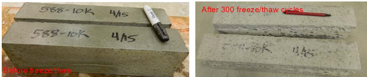
Figure D6- Visual appearance of specimens before and after freeze and thaw test for W.R Meadow SEALTIGHT 588-10K (Mix #6)
