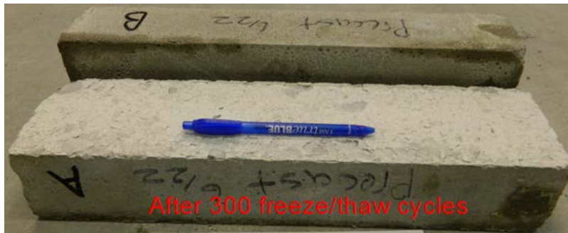
Figure D10- Visual appearance of specimens after freeze and thaw test for Euclid Euco Precast Grout (Mix #20)
