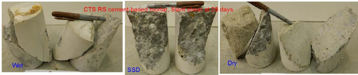
Figure G9-Failure mode of slant shear bond test at 28 days for CTS rapid-set cement-based mortar with different substrate surface moisture conditions (#54)
