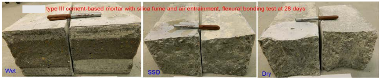
Figure F3-Failure mode of flexural bond test at 28 days for type III cement-based mortar using natural river sand, AEA, and different substrate surface moisture conditions (#47)
