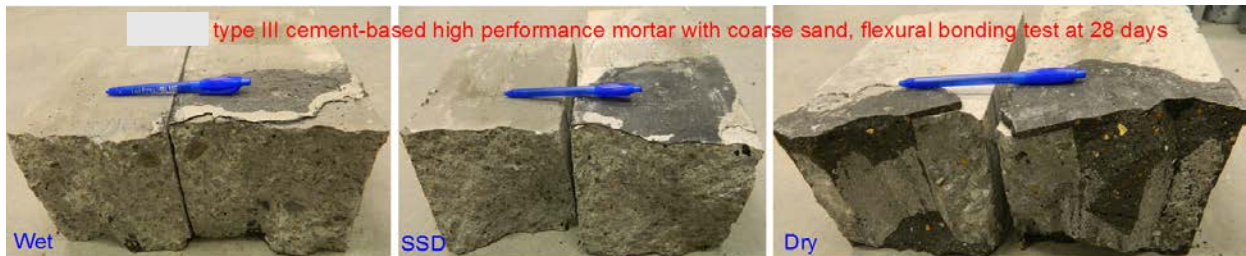
Figure F4-Failure mode of flexural bond test at 28 days for type III cement-based high performance mortar using natural river sand and different substrate surface moisture conditions (#48)
