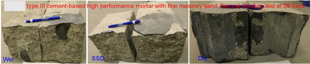
Figure F6-Failure mode of flexural bond test at 28 days for type III cement-based high performance mortar using fine masonry sand and different substrate surface moisture conditions (#50)
