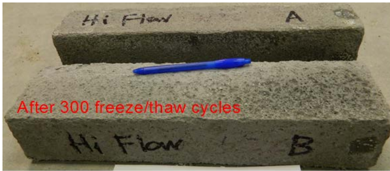
Figure D13- Visual appearance of specimens after freeze and thaw test for Euclid Hi-flow Grout (Mix #23)
