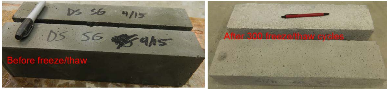
Figure D5 - Visual appearance of specimens before and after freeze and thaw test for Dayton Superior Sure-Grip High Performance Grout (Mix #5)
