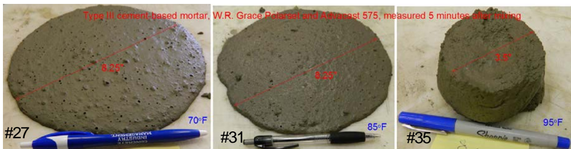
Figure E2-Spread of mini slump test for type III cement-based mortars (#27, #31, and #35) using W.R. Grace Polarset (accelerator) and Adva-Cast 575 (superplasticizer) at different temperatures
