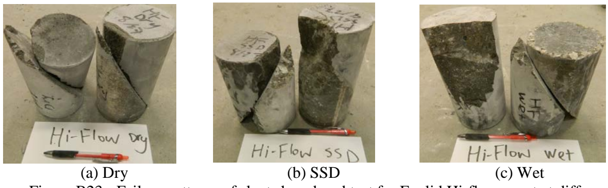
(a) Dry (b) SSD (c) Wet Figure B23 - Failure patterns of slant shear bond test for Euclid Hi-flow grout at different substrate surface moisture conditions at normal temperature (73°F) (Mix #23)
