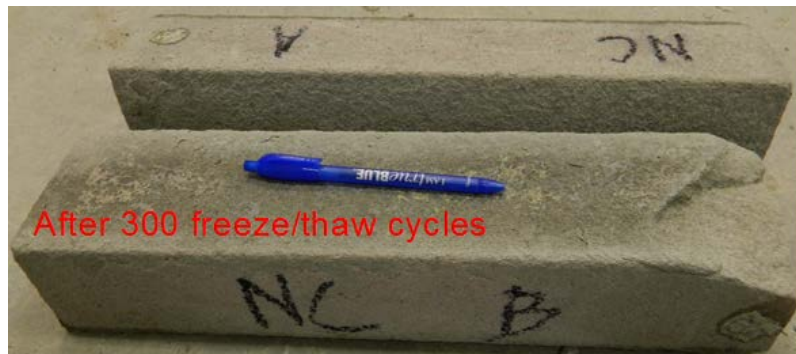
Figure D11- Visual appearance of specimens after freeze and thaw test for Euclid NC Grout (Mix #21)
