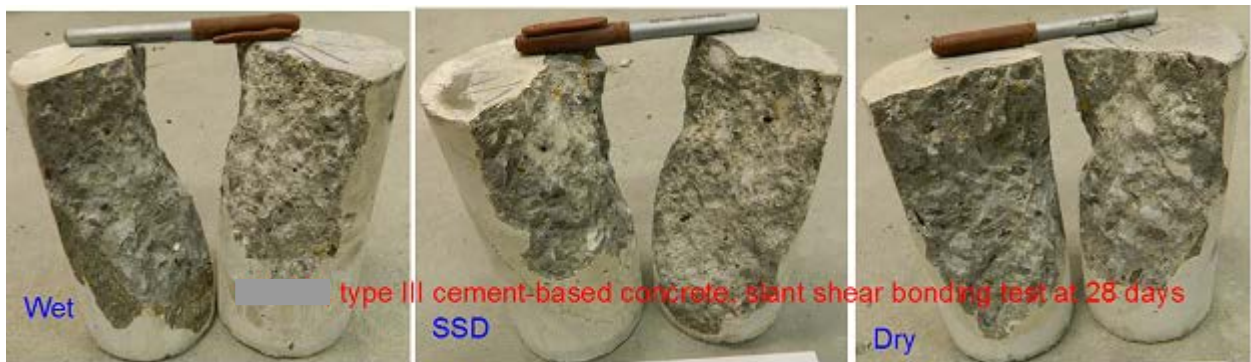
Figure G8-Failure mode of slant shear bond test at 28 days for type III cement-based concrete with different substrate surface moisture conditions (#52)
