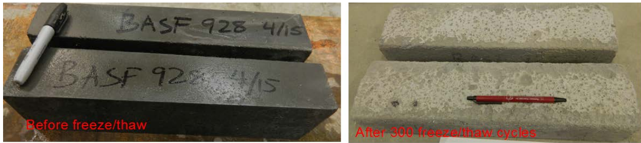
Figure D1- Visual appearance of specimens before and after freeze and thaw test for BASF Masterflow 928 (Mix #1)
