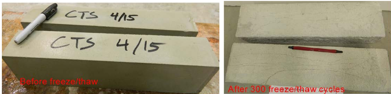
Figure D7- Visual appearance of specimens before and after freeze and thaw test for CTS Rapid Set CEMENT ALL Grout (Mix #7)
