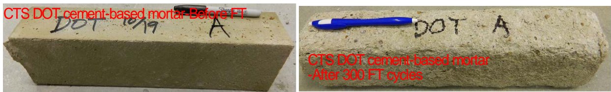
Figure H9-Visual appearance of freeze and thaw test specimens for CTS DOT cement-based mortar (#55)
