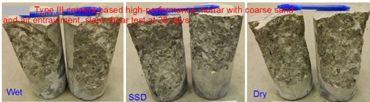
Figure G5-Failure mode of slant shear bond test at 28 days for type III cement-based high performance mortar using natural river sand, AEA, and different substrate surface moisture conditions (#49)
