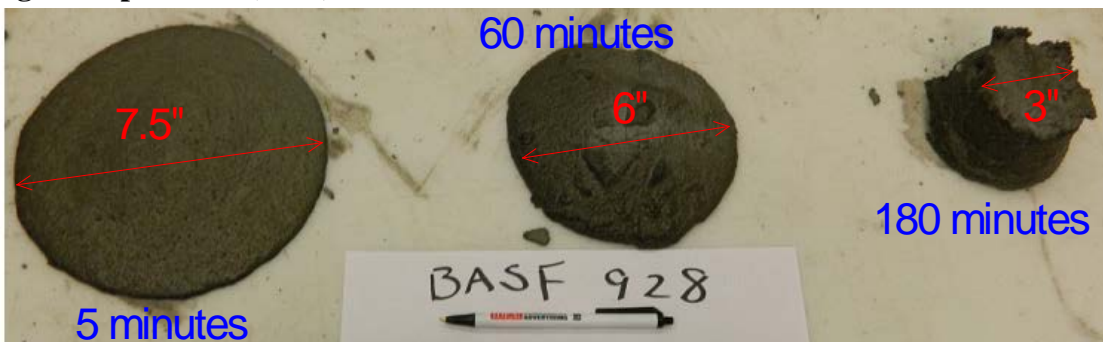
Figure C35 - Spread of mini slump test for BASF Masterflow 928 Grout at different time at high temperature (95°F) (Mix #1)
