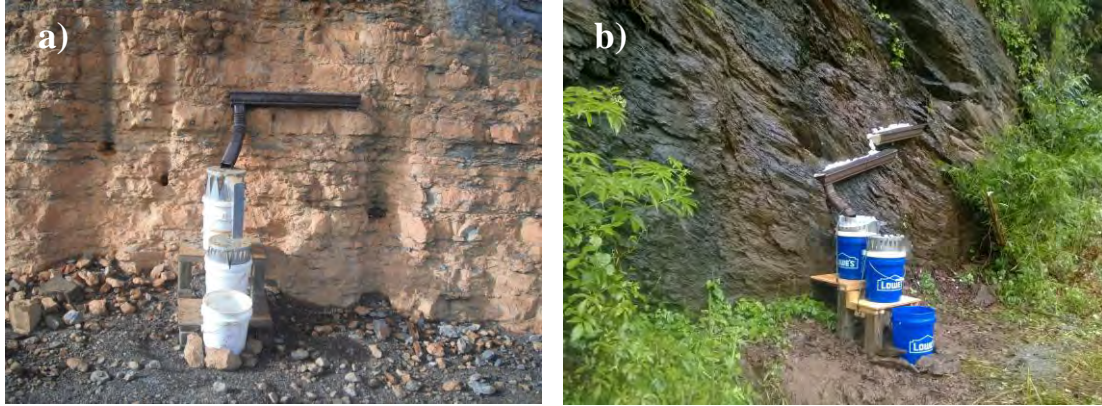
Figure 2.2. Photos of Pinson et al. (2003) flow divider buckets for passive runoff collection at the monitoring sites: a) Nashville 2 (N2) and b) Ocoee 1 (O1).
