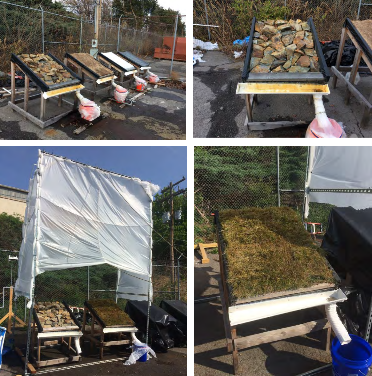
Figure 3.2. Photos of the experiment set-up on Middlebrook Pike, Knoxville, Tennessee showing Anakeesa Formation rock treatment trays ( upper right photo – exposed rock and lower right photo – soil/grass), and the rainfall simulator ( lower left photo ).
