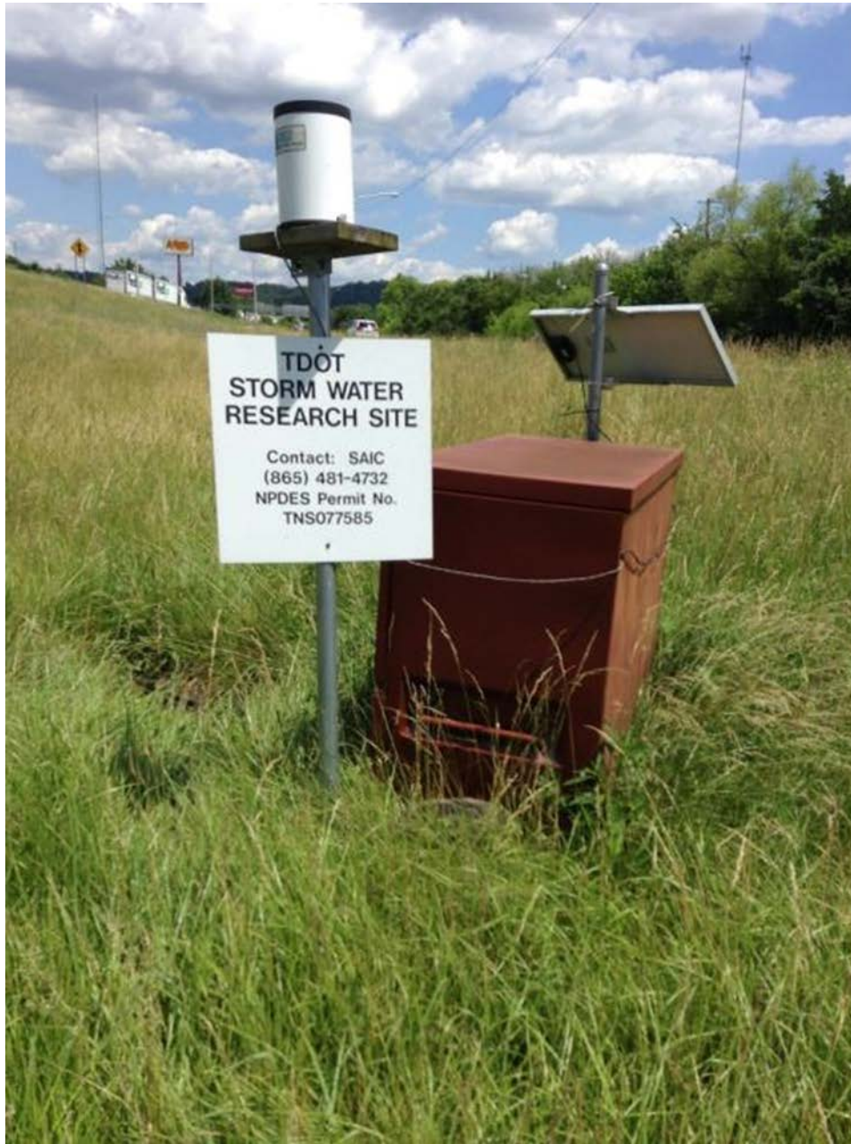
Figure B.1. Site RO2 security box, rain gage, and solar panel.
