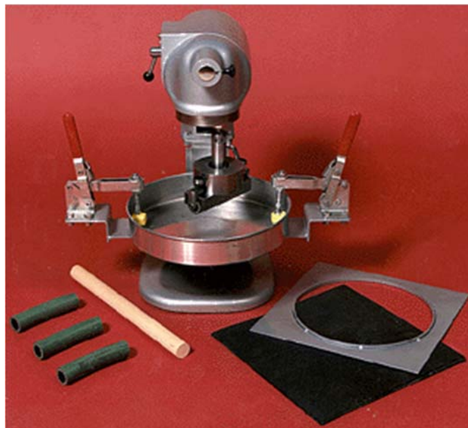
Figure 1. Wet track abrasion tester – Hobart N-50 (Mastard Limited).
