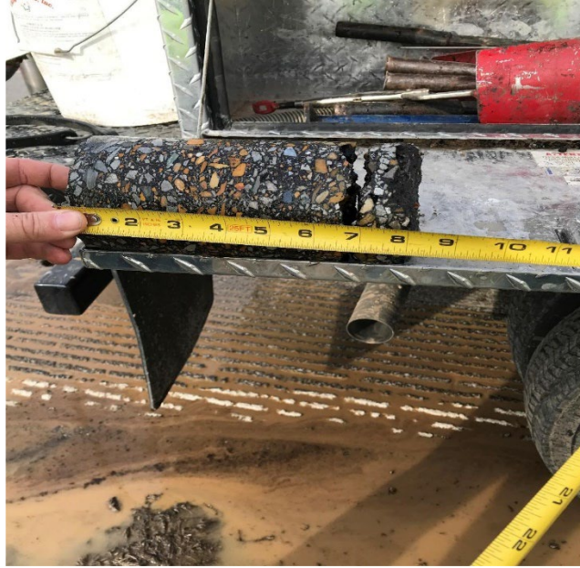
Figure C 9 Core #11 (8 ¼") was drilled at 5.1 mile and corresponds to sample # 6
