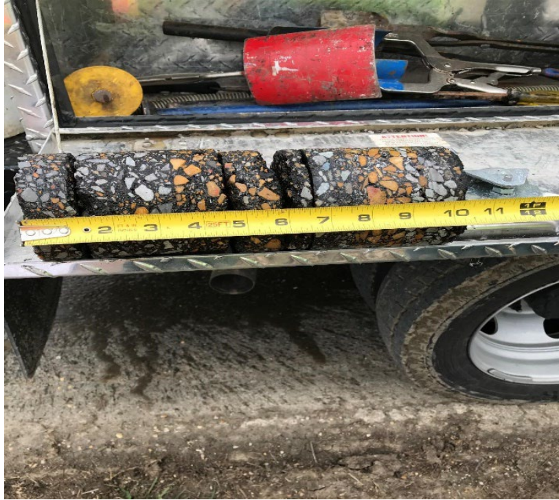
Figure C 3 Core#5 (10 ½") was drilled at 2.1 mile and corresponds to Sample # 3
