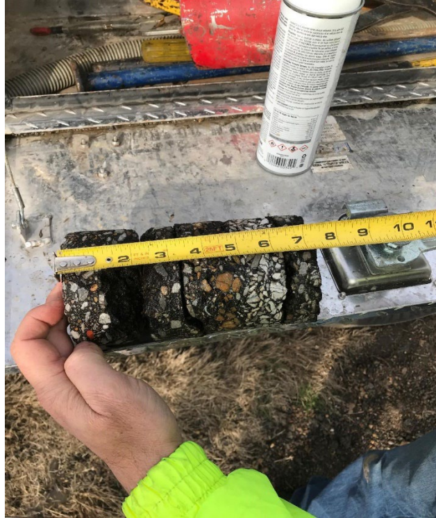
Figure C 7 Core #9 (8 3/4") was drilled at 4.0 mile and corresponds to sample # 5
