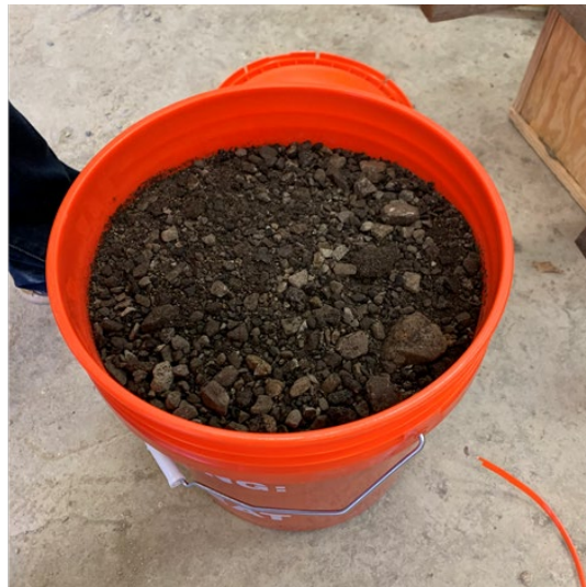
(b) Reclaimed Pavement Materials
