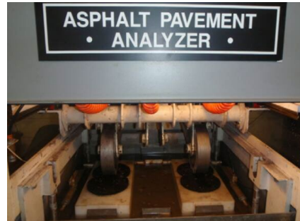
Figure 4-36. Setup for Hamburg wheel test
