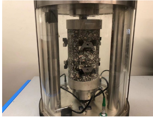
Figure 4-20. Dynamic modulus test
