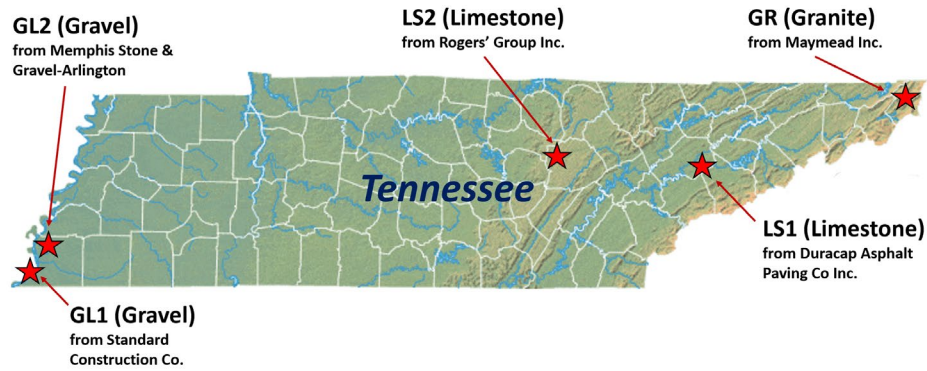
Figure 4-1. Five types of aggregate sourced from different quarries in Tennessee
