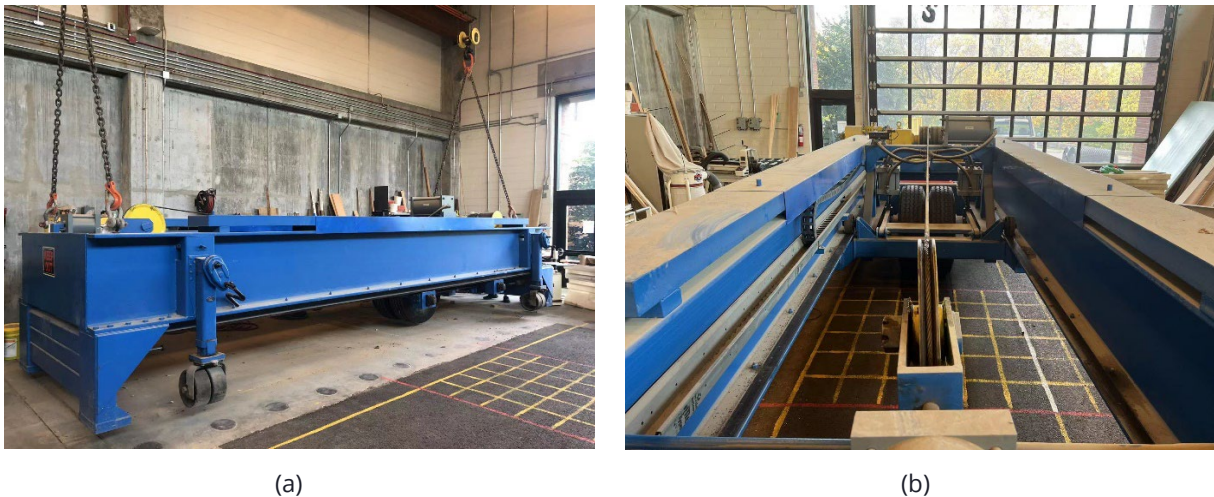
Figure 3-1. The accelerated pavement testing (APT) facility
