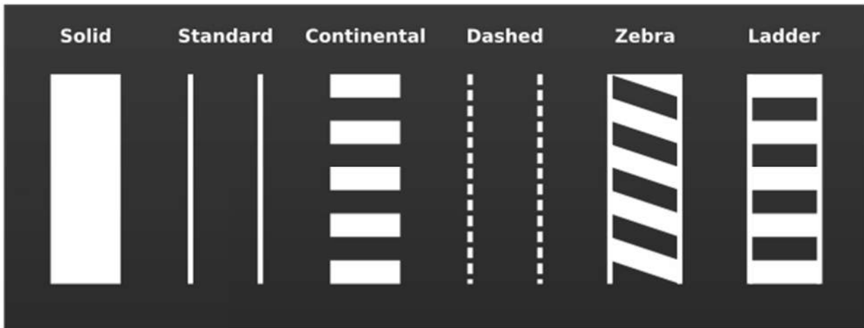
Figure 21 - Crosswalk Marking Examples
