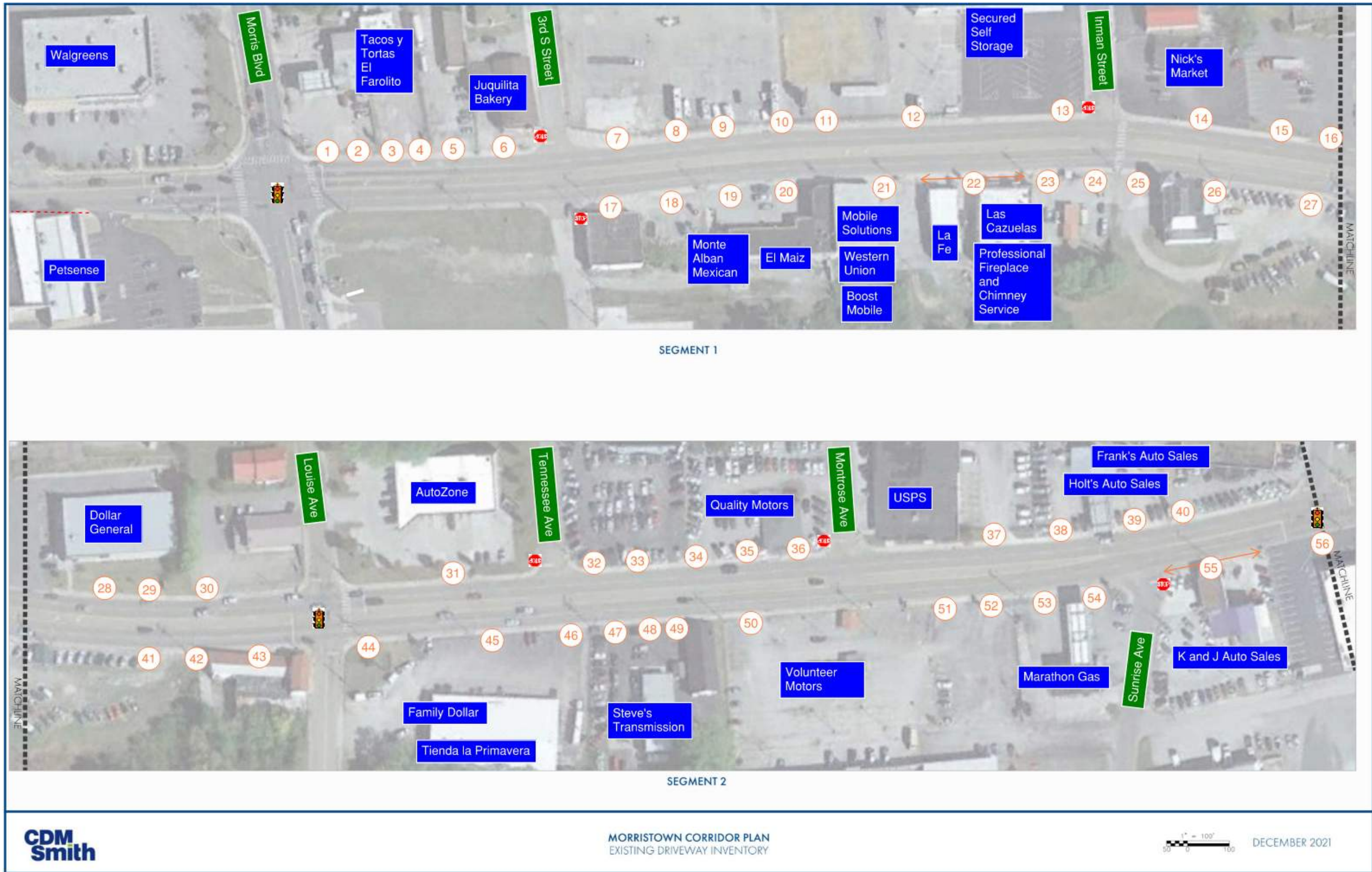
Figure 13 - Existing Driveway Inventory Sheet 1 of 3 (Segments 1 and 2)
