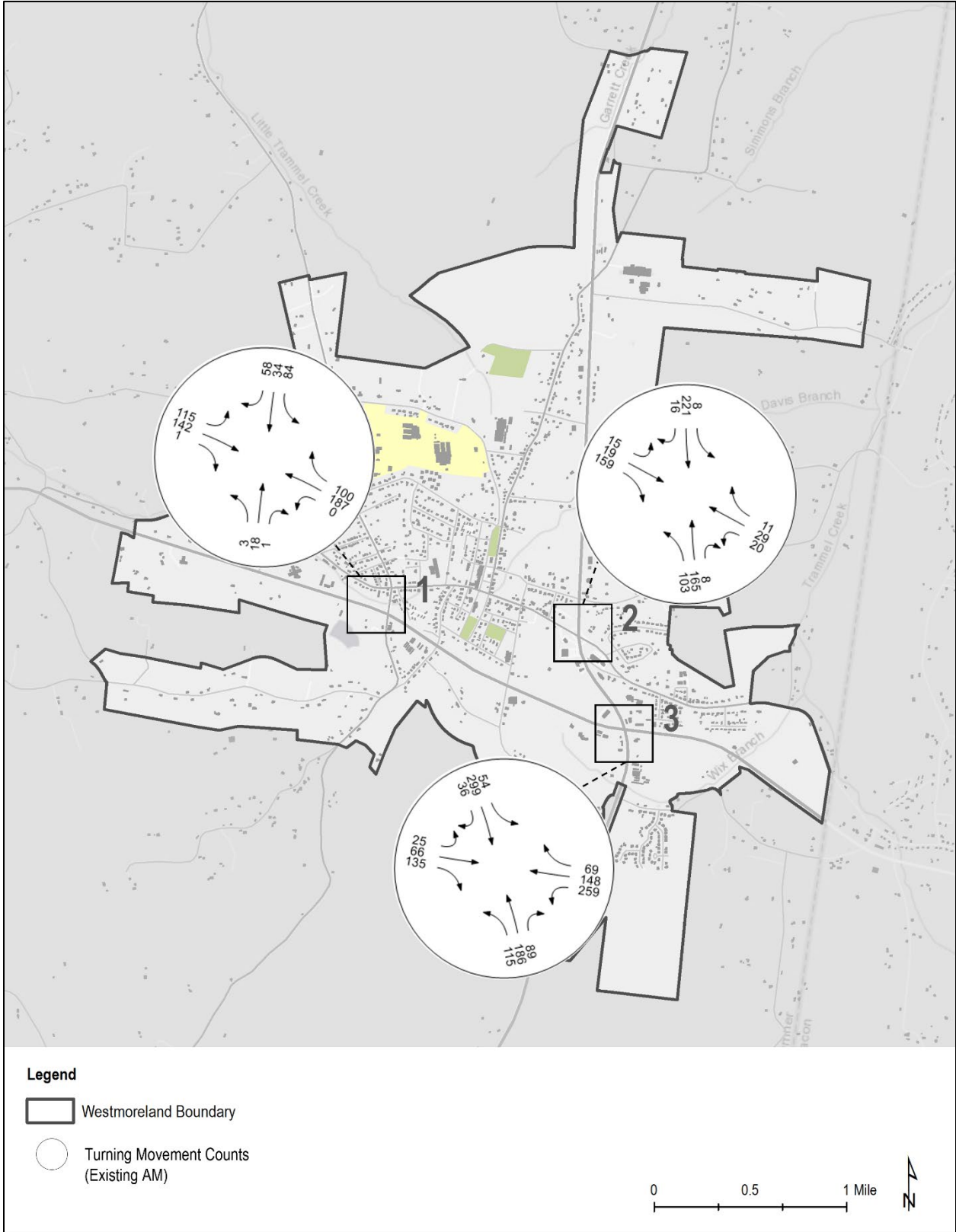
Figure 2-7. Existing Peak Hour Turning Movement Counts (AM)
