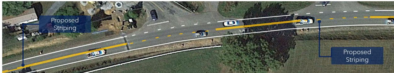
Figure 5-2 Pavement Marking Improvements at Pleasant Grove Road and Broyles Lane
