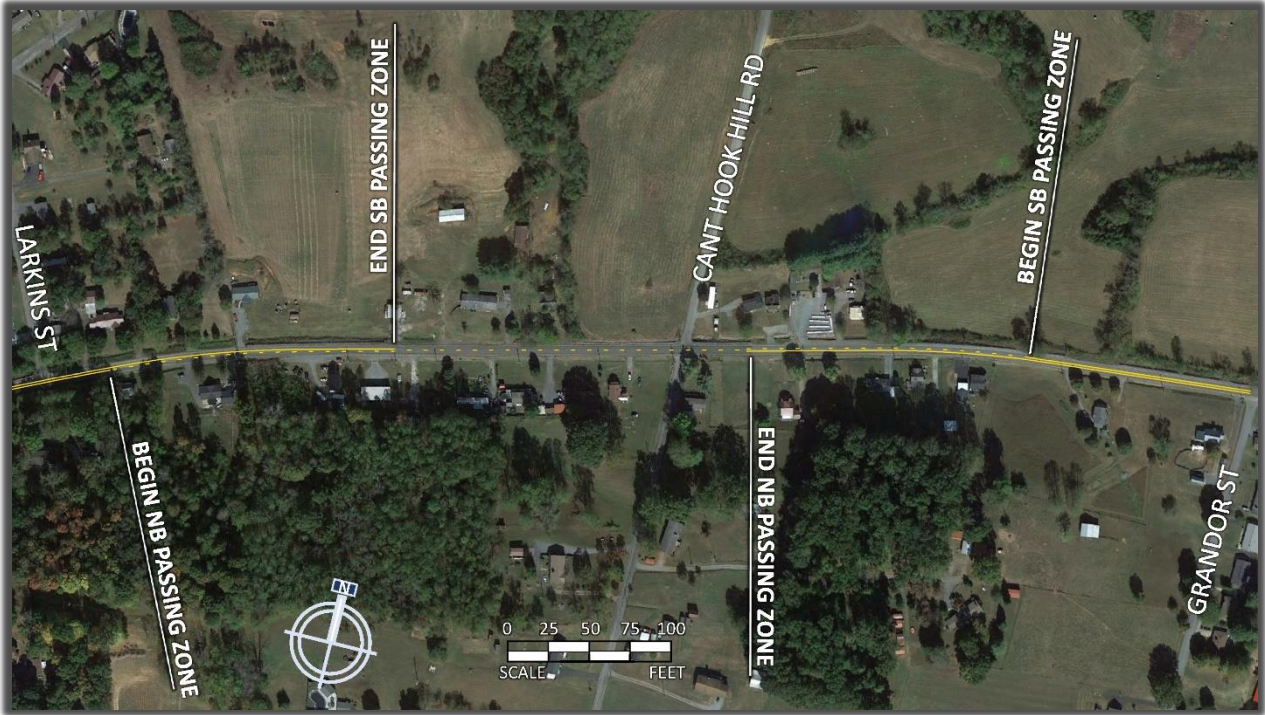
Figure 2-9 Passing Zone at Cant Hook Hill Road
