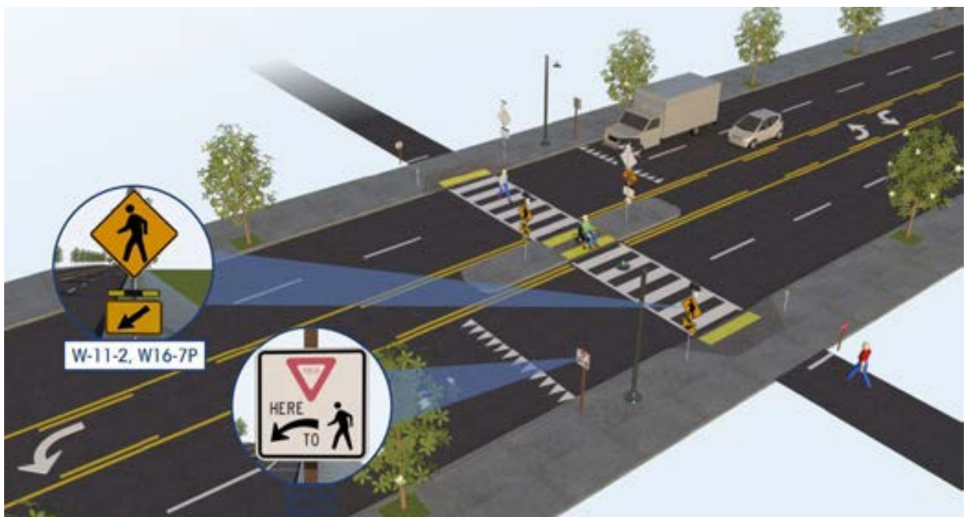
Clearly marked pedestrian crossings are essential part of first and last mile connections that help transit riders comfortably and safely to and from their ultimate destination. (Source: Rapid Rectangular Flashing Beacon from the Federal Highway Administration). Image URL: https://safety.fhwa.dot.gov/ped_bike/step/docs/TechSheet_RRFB_508compliant.pdf
