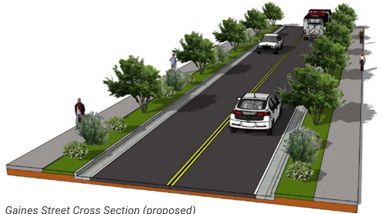
Gaines Street Cross Section (proposed)
