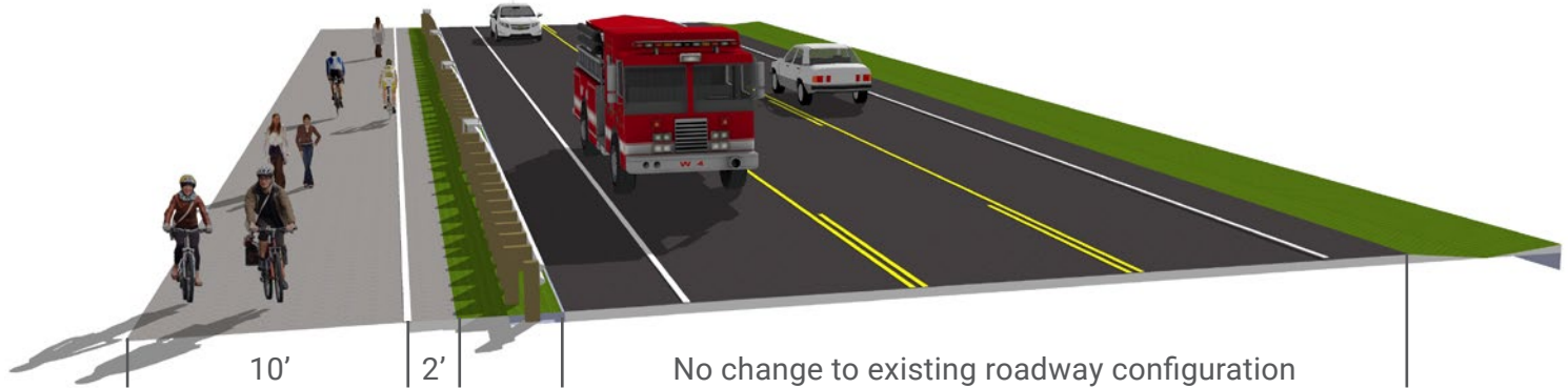
Figure 4.19: Roaring River Park Greenway Cross Section - Off-Street
