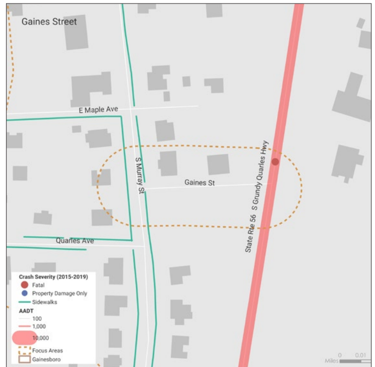
Figure 2.7: Crash locations and severity, and traffic volumes within the SR-56/Gaines Street focus area. One fatality recorded at this location between 2014-2019. Source: TDOT.
