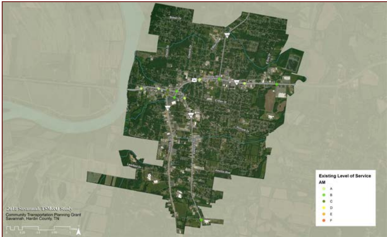
Figure 3.1 Existing Level of Service – AM Peak
