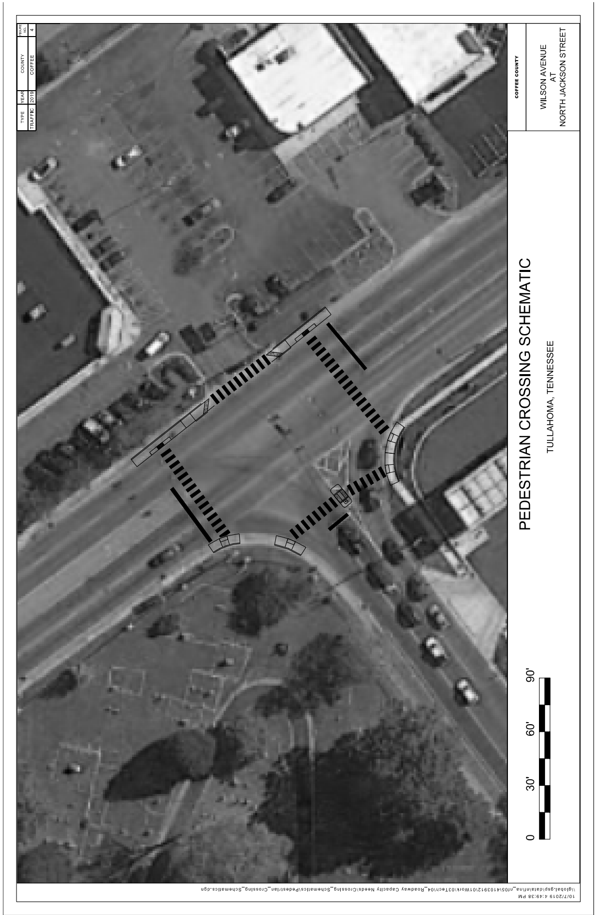
Figure 4-10. Crossing Schematic – US-41A/North Jackson Street at SR-55/Wilson Avenue
