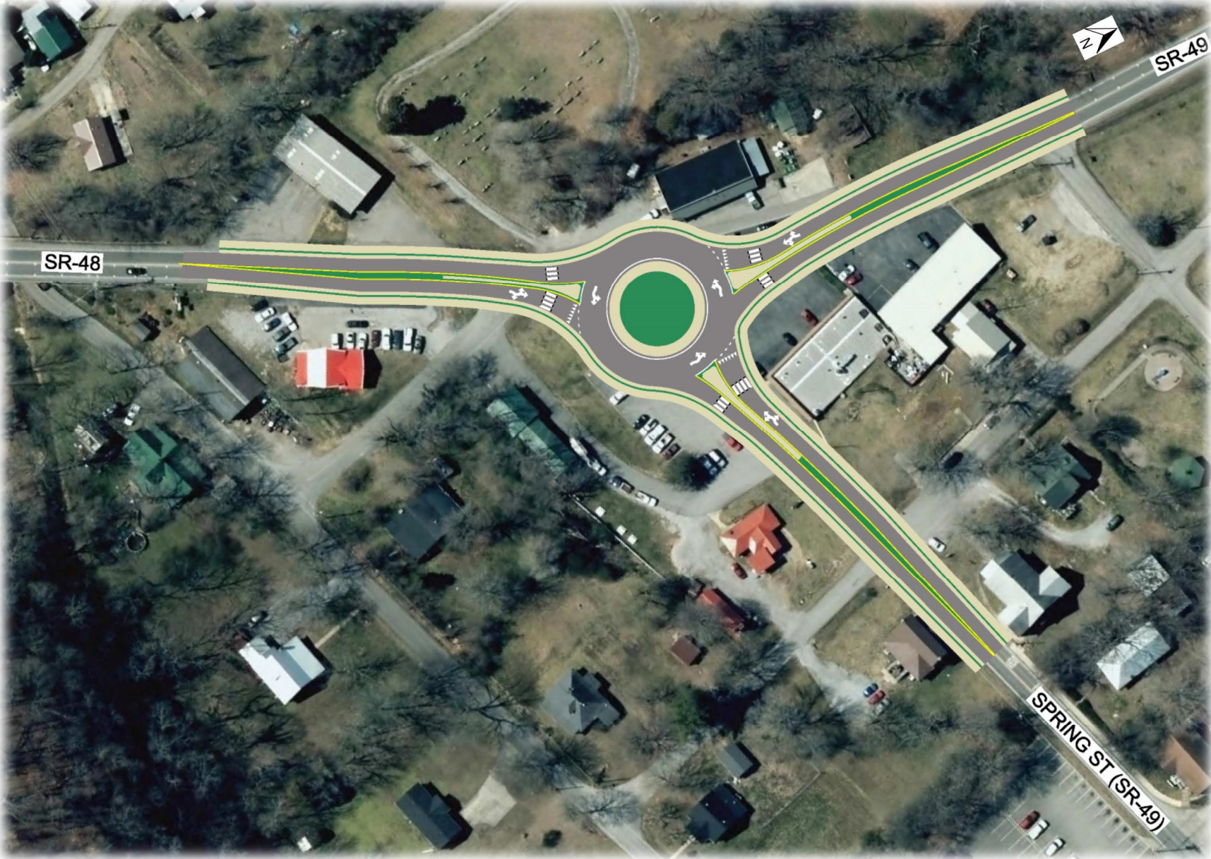
PROPOSED ROUNDABOUT AT SR-48 AND SPRING STREET
