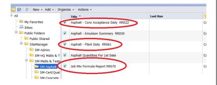
The "SM-Asphalt" folder includes a "Job Mix Formula" report to see needed asphalt mix design data. An "Asphalt - Plant Daily" report that will eventually replace the existing DT form. And the "Asphalt – Core Acceptance Daily" report is also ready for future use.
