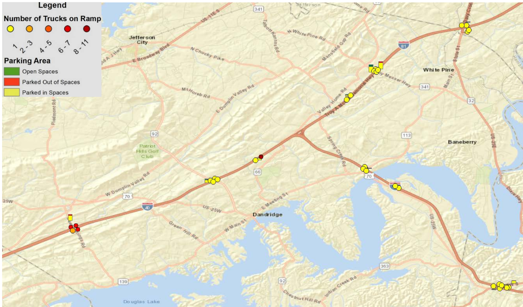
FIGURE A11 illegal ramp parking with volume to capacity ratio on Interstate 40 near Dandridge, Tennessee
