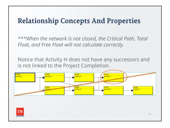
\*\*\*When the network is not closed, the Critical Path, Total Float, and Free Float will not calculate correctly.
