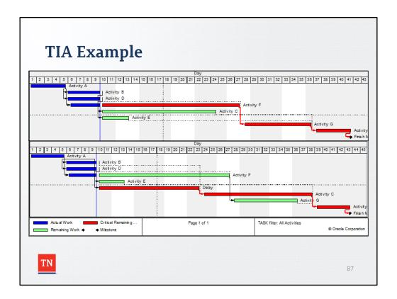
In summary, the 14-day delay to Activity C resulted in an overall delay to the completion of 2 days. Additionally, the Critical Path changed from Activities A-F-G-H to Activities A-B-C-H.
