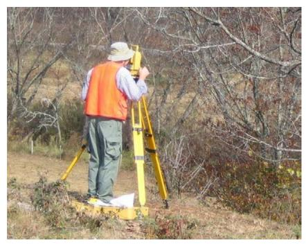
Figure 2-2. Using a total station to survey a stream.
