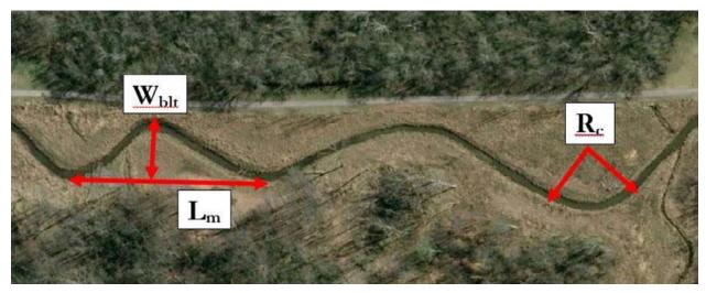
Figure 3-4. Typical pattern measurements.
