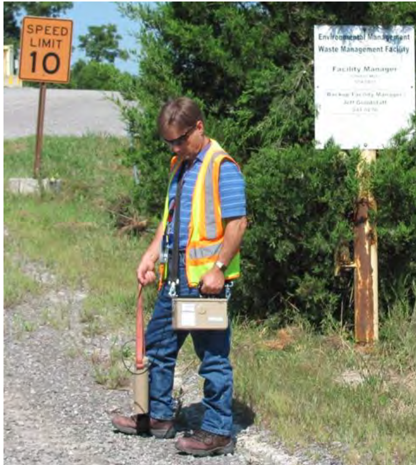
TDEC personnel perform an ambient gamma survey of the Haul Road (TDEC photo)
