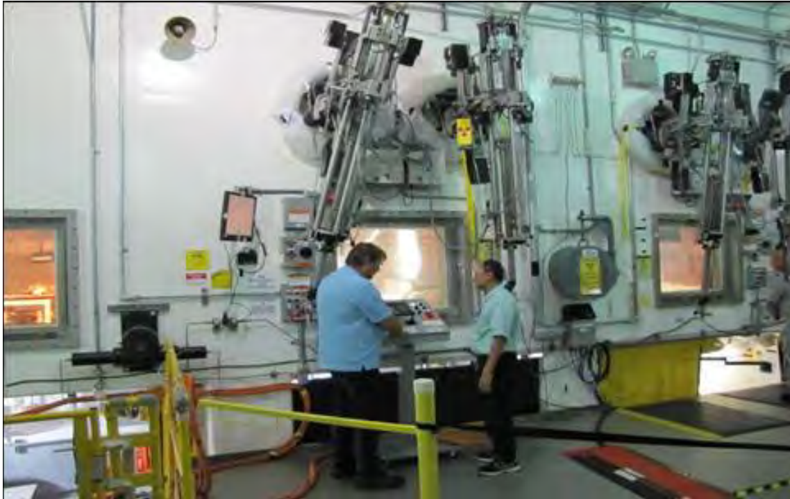
Operation of manipulator arms at TWPC (DOE photo)
