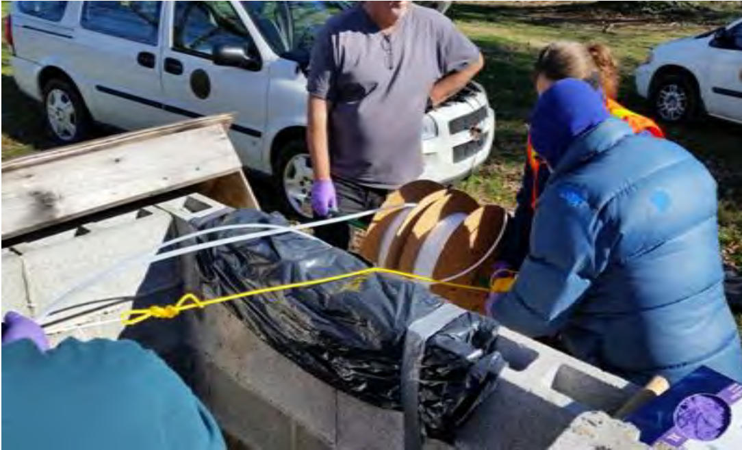
TDEC personnel sample a residential well using a peristaltic pump (TDEC photos)
