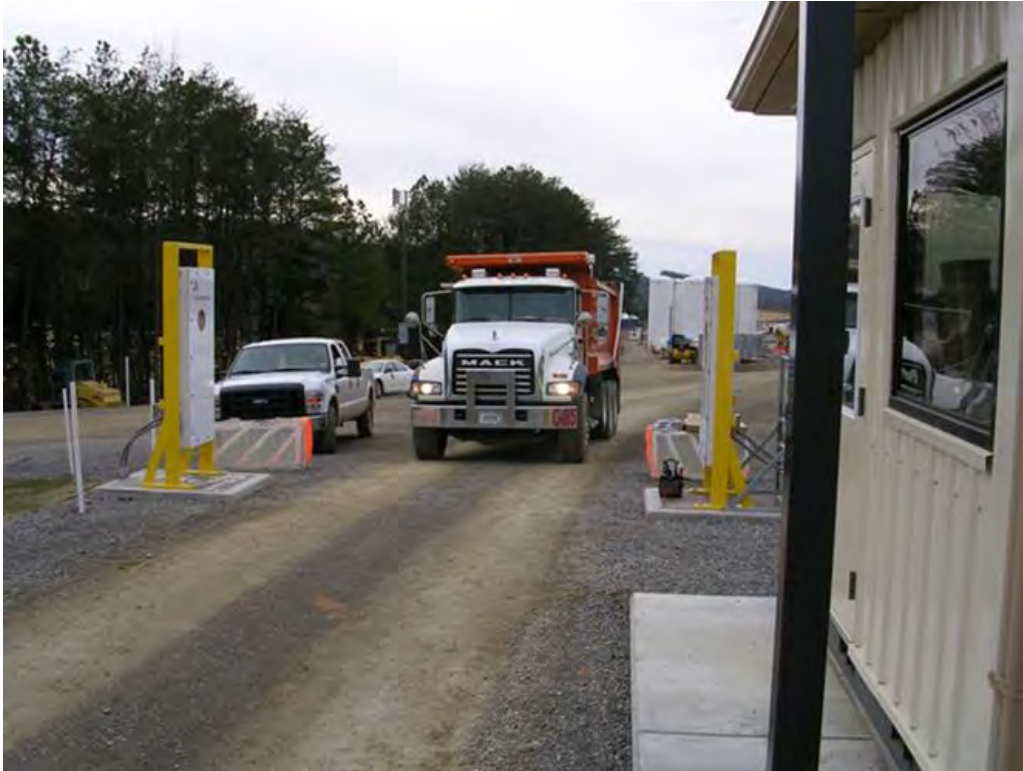
Truck hauling waste to EMWMF passes through the radiation portal monitor (TDEC photo)
