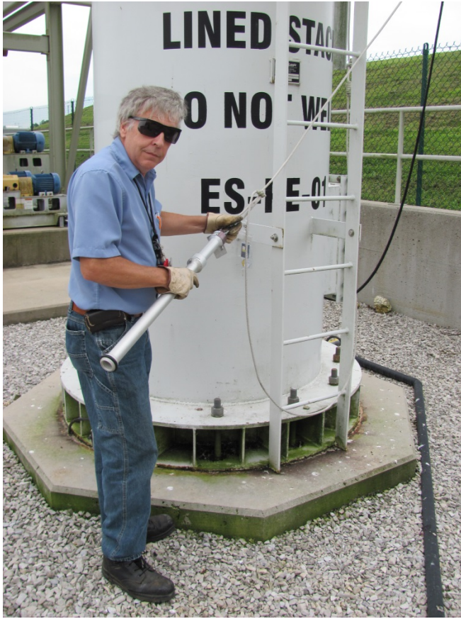
Gary Riner uses a rope and pulley system to deploy a gamma radiation logger on the main stack at the Spallation Neutron Source. (TDEC Photo)
