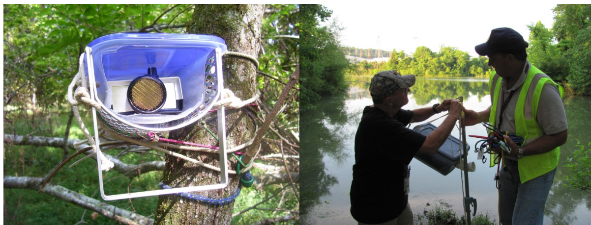
Left, bat call recorder deployed on a tree. The recordings are analyzed with computer software to identify bats by their echolocation calls. Right, Gerry Middleton and Wes White deploy another at a pond on the DOE reservation. (TDEC photos)
