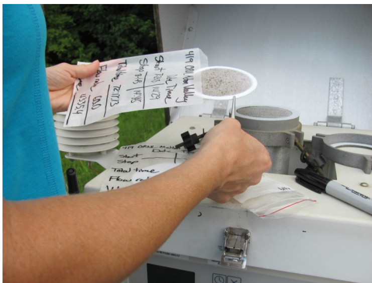
RadNet sample media being collected for shipment to EPA labs. (TDEC photo)
