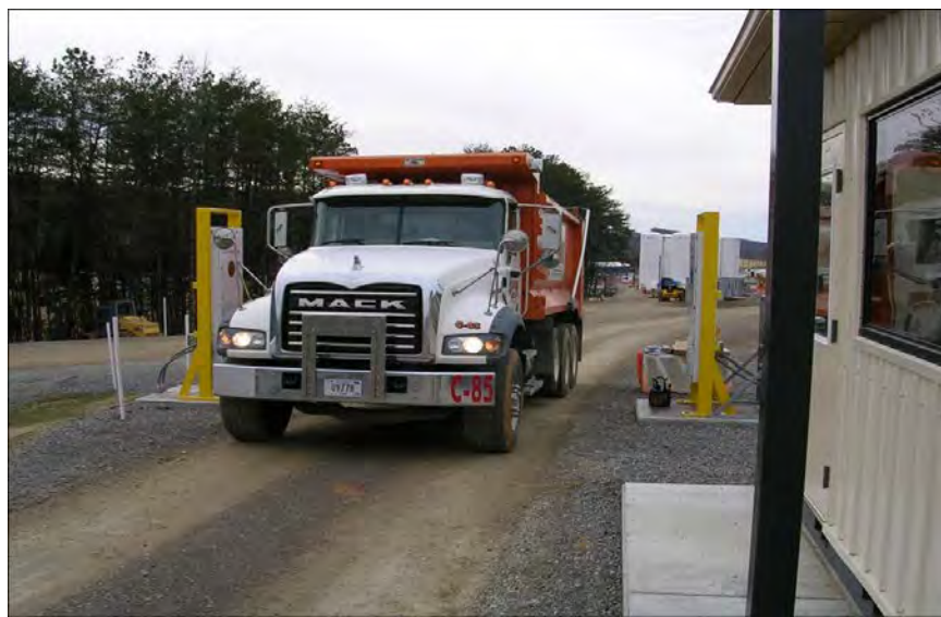
Figure 2.2.2.2.1 TDEC portal monitor at EMWMF
