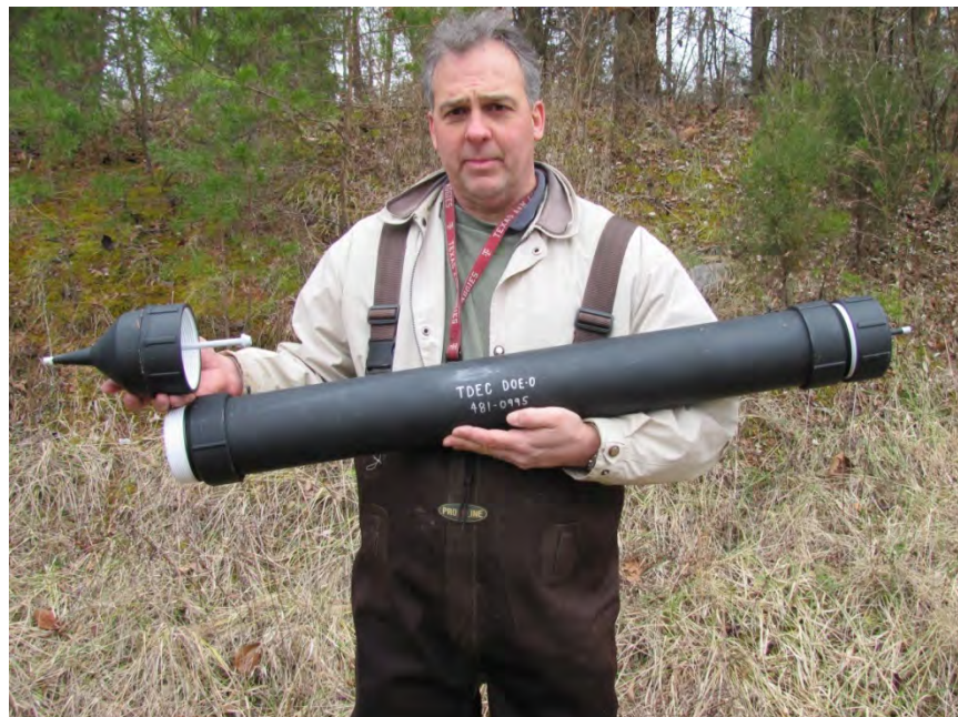
Figure 2.1.6.2.3 Photo of sediment trap
