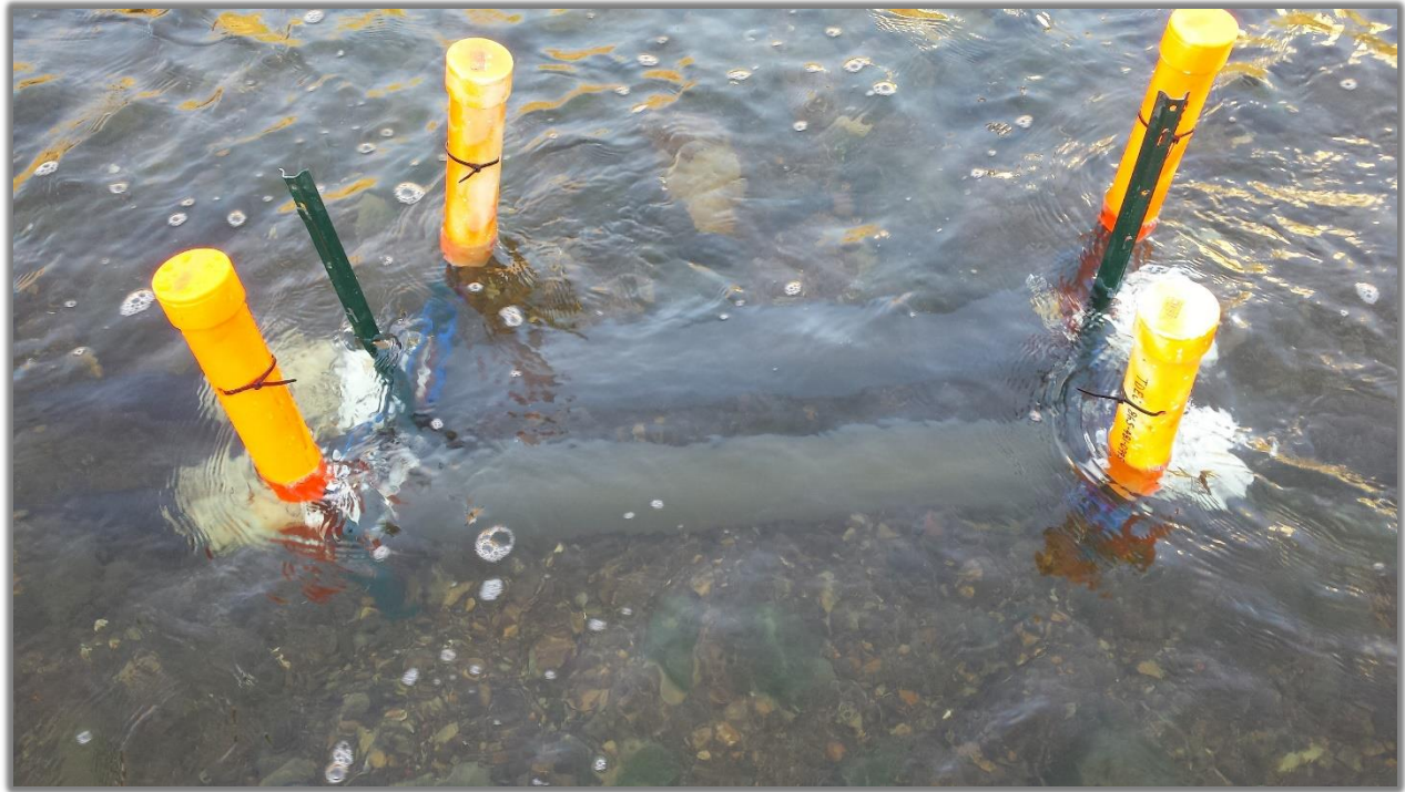
Figure 8.1.8.1 Tandem sediment trap installation in East Fork Poplar Creek (EFPC)
