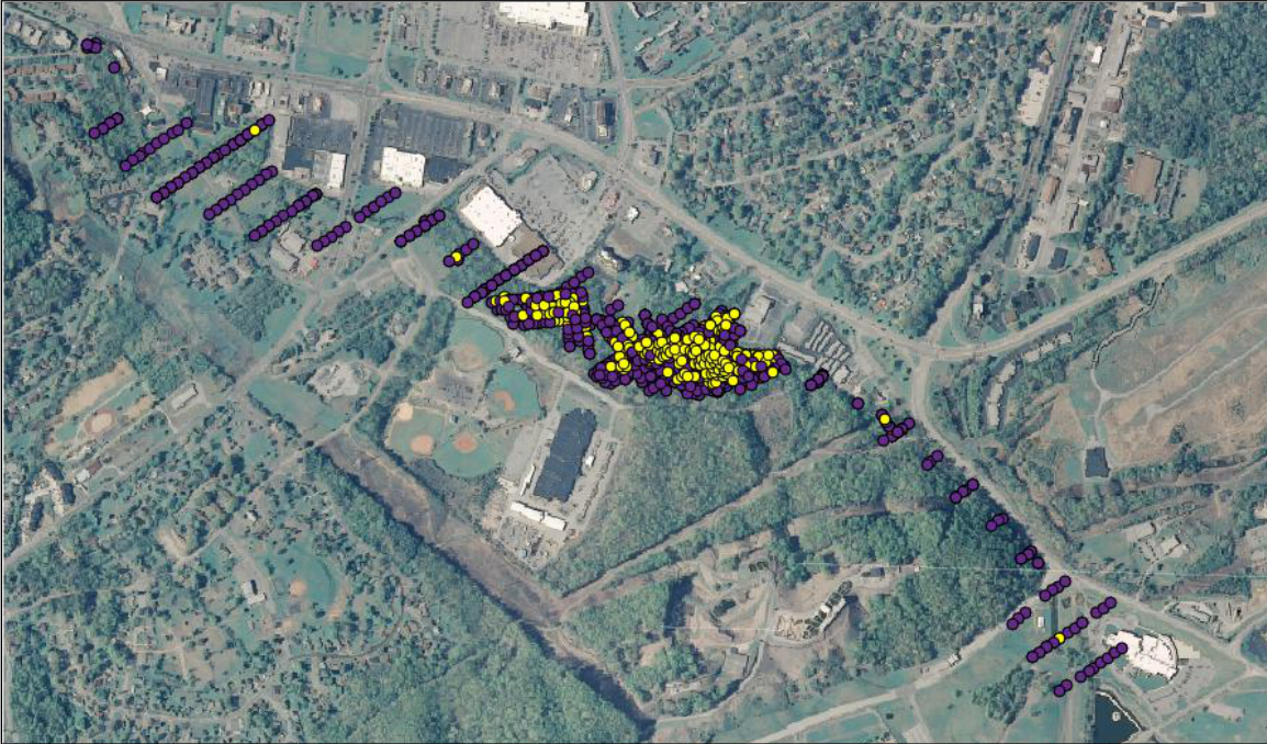
Figure 6: OREIS Database Pre-Remediation Hg Samples (Yellow Circles = >100 ppm Hg; Purple Circles = <100 ppm Hg)
